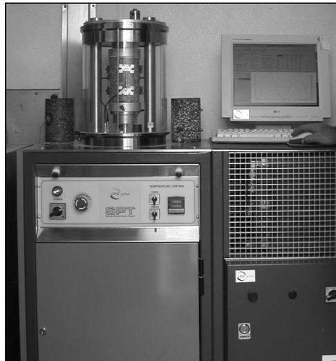
**Figure 1. Simple Performance Test (SPT) Device in FHWA Mobile Asphalt Laboratory**
