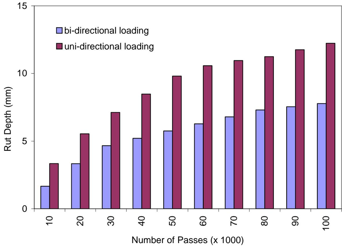
**FIGURE 2** A comparative illustration of respective rut measurements resulting from uni- and bi-directional modes of loading.
