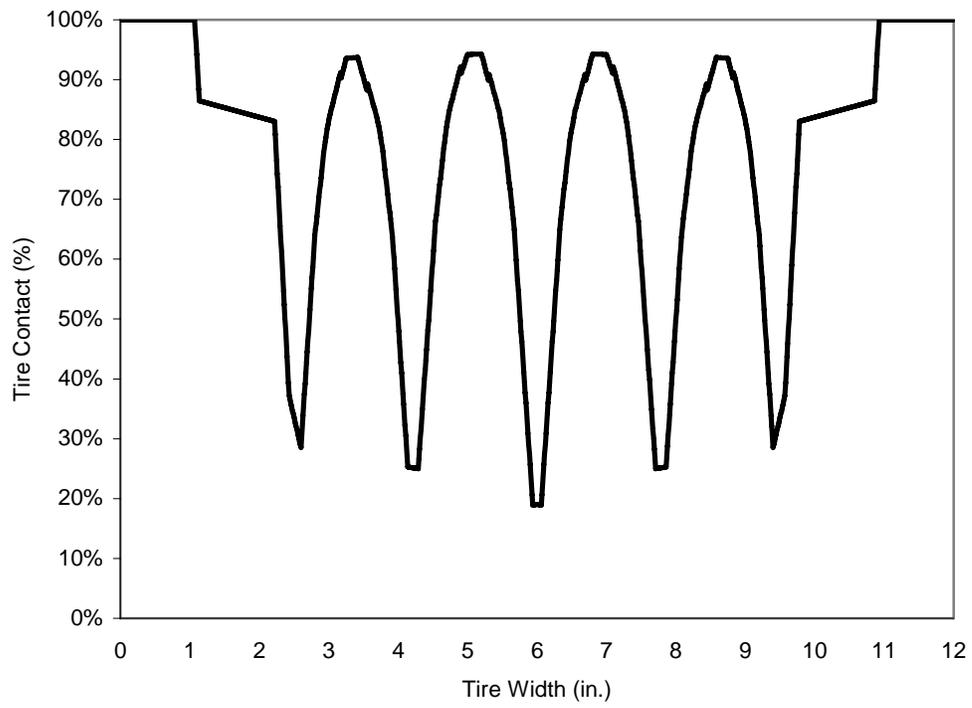
**FIGURE 7** Amounts of tire-pavement contact as measured along the tire width
