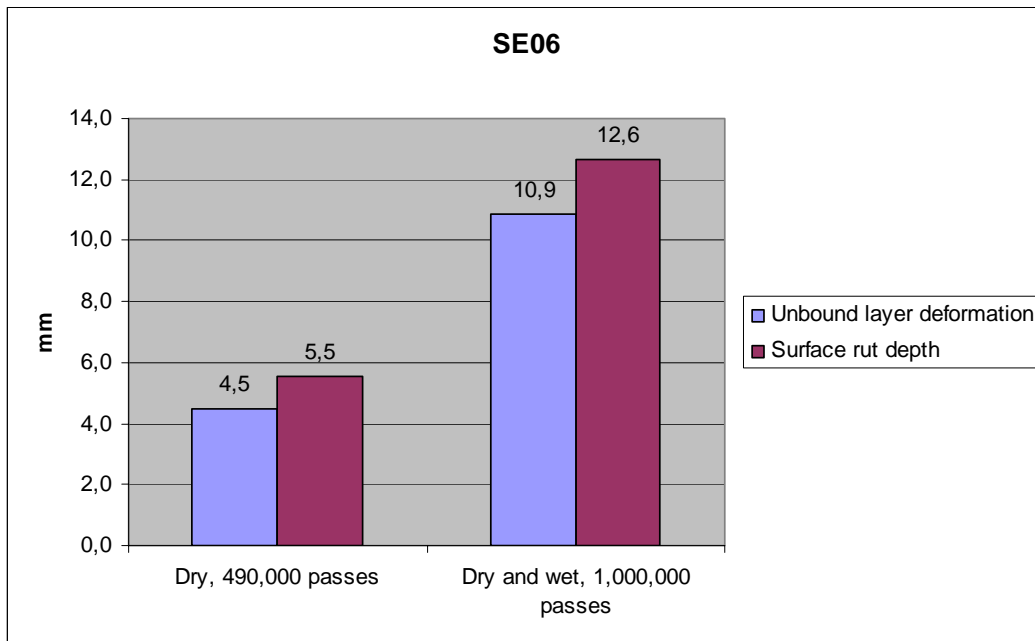
Figure 30 Total deformation of unbound layers compared to pavement surface rut depth. Unbound layers include base, sub-base, and the upper 300 mm of the subgrade.
