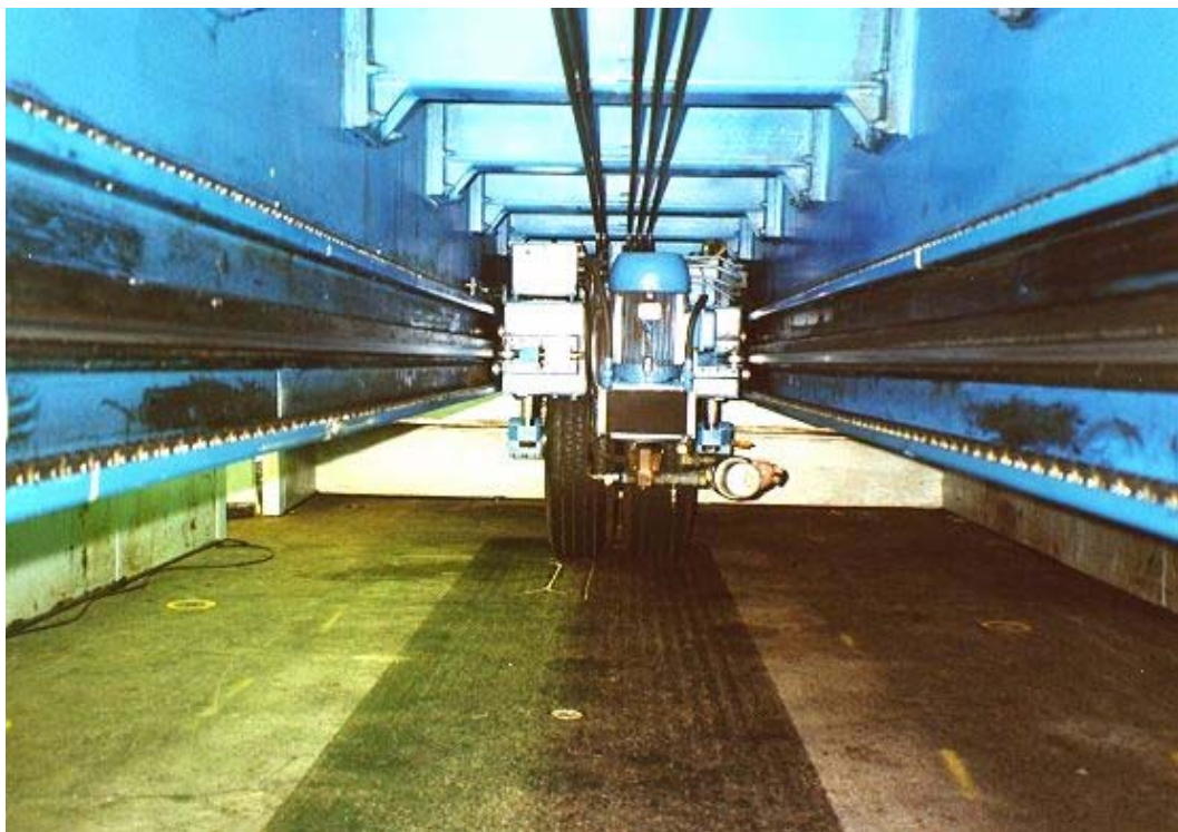
Figure 3 Inside view of test-carriage and loading wheel.
